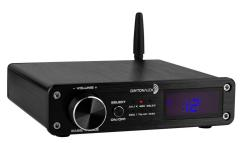
Highly efficient class-D amplifier topology delivers an uncolored, pleasing audio experience. The DTA-PRO offers an astonishing 100W of power that will drive even the most demanding of speakers. In addition to a powerful stereo amplifier, the DTA-PRO also features a line level output for a powered subwoofer. Capable of producing a tight, wallshaking listening experience, the DTA-PRO's 3 VRMS sub output provides a powerful, driving low-end response.
