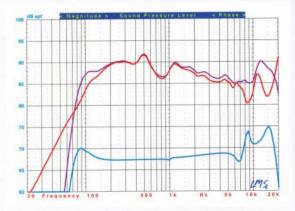
**EPIQUE CBT24 w EQ (purple)** +3.53/-3.16 dB, 200 Hz to 10 kHz; -3 dB @ 88 Hz, -6 dB @ 79 Hz; impedance minimum 4.52 ohms @ 625 Hz, phase angle -37.39° @ 208 Hz; sensitivity 88 dB, 500 Hz to 2 kHz.
