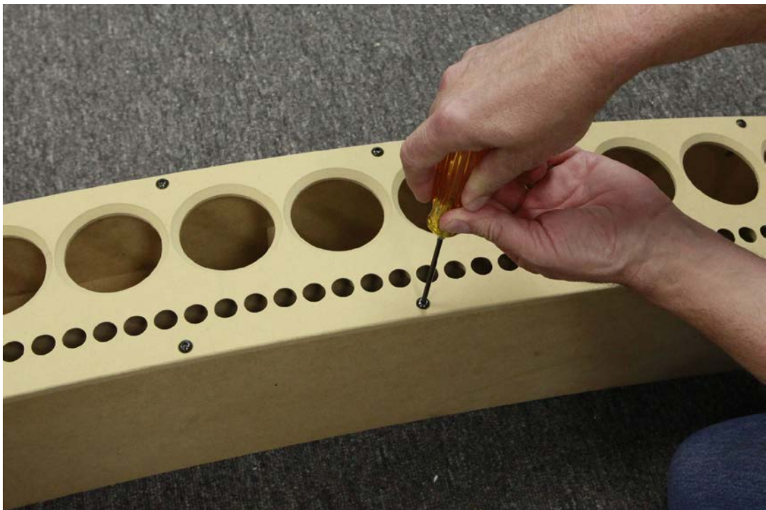
Fig. 4. CBT36 cabinet showing front panel being unscrewed.
