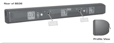
Step 2: Identify mounting location and attach wall bracket to the wall using supplied drywall screws. Do not use nails. Attach one end first then pivot until bubble is level. Mark holes and install remaining screws. When using the supplied "Wall Dog" screws it is not necessary to locate a wall stud.
