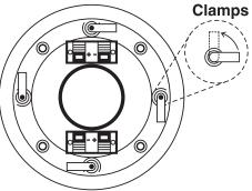
CAUTION: Do Not Over-Tighten the Clamps. Too much torque may snap off the lug and the speaker will not seat securely. A snug fit is all that is necessary to assure proper performance.
