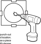
hole and rotate the wire in a complete circle to check for obstructions. If the wire hits a stud on either side, reposition your template to the left or right and drill a new hole at the center, then repeat the test until a clear area is located.
