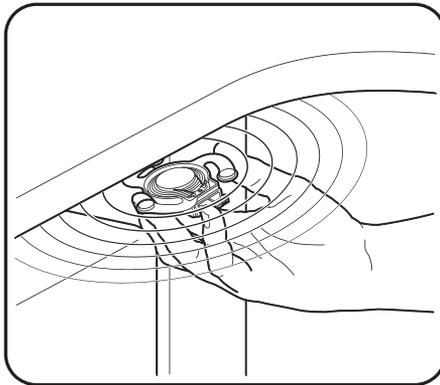
***NOTE: Before permanently attaching the Sound Exciters, test the placement for optimal sound reproduction.***
