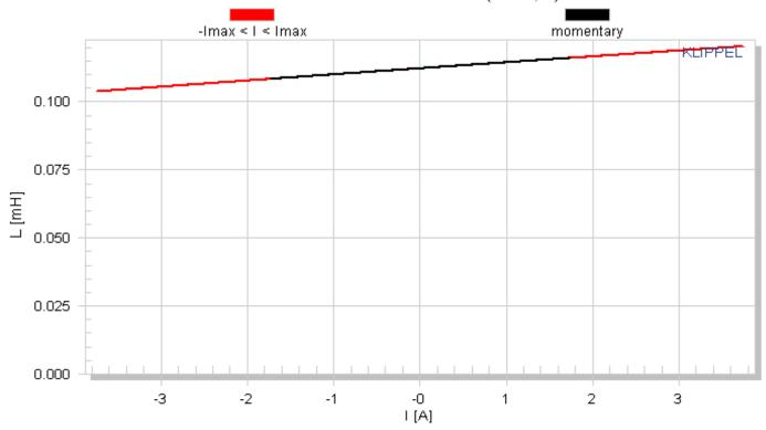
The inductance components Le (x) and BI(i) of most drivers have a strong asymmetric characteristic. If the voice coil moves towards the back plate the inductance usually increases since the magnetic field generated by the current in the voice coil has a lower magnetic resistance due to the shorter air path.
