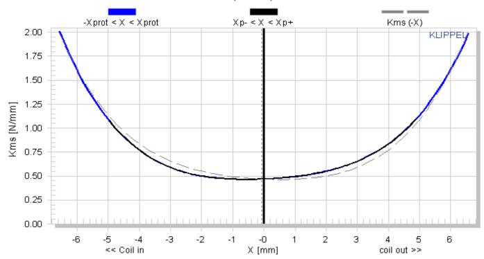
The stiffness KMS(x) describes the mechanical properties of the suspension. It's inverse is the compliance CMS(x)
