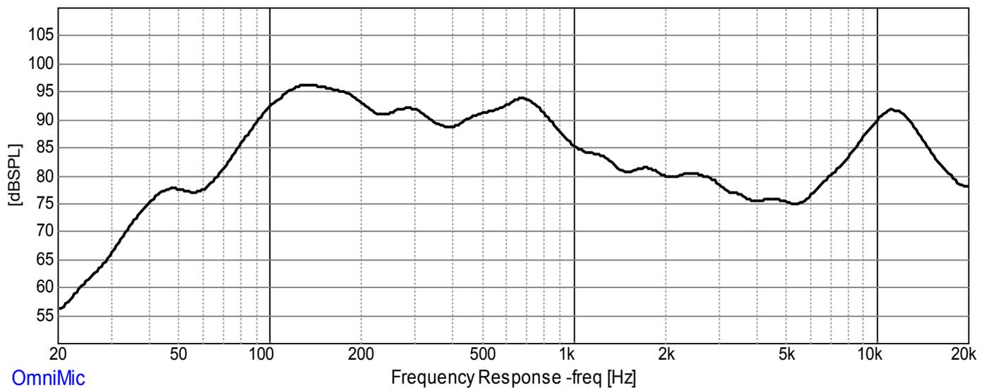
1/3rd octave smoothing - measurement taken with transducer adhered off-center on a 12" x 12" x 1/2" foam core board in an infinite baffle setup.
