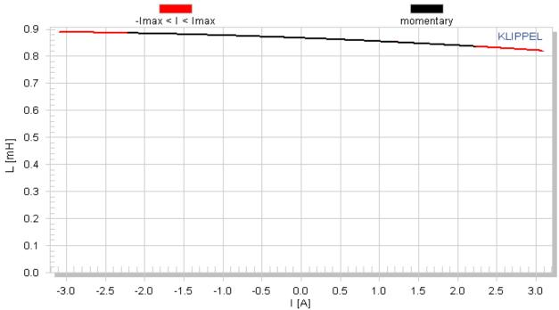
The inductance components Le (x) and Bl(i) of most drivers have a strong asymmetric characteristic. If the voice coil moves towards the back plate the inductance usually increases since the magnetic field generated by the current in the voice coil has a lower magnetic resistance due to the shorter air path.
