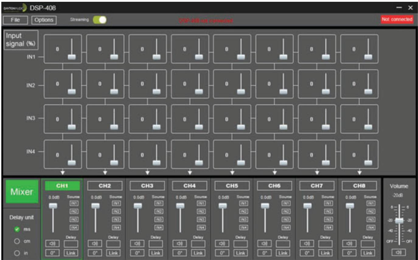
1. **Mixer:** The user can select what percentage of each input is routed to each output simply by using the sliders.
