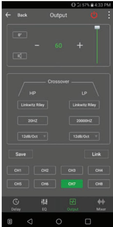
1. **Phase Control:** The “0°” button can be pressed to invert the phase 180°, to revert back, press the same button again, which is now labeled “180°”.
