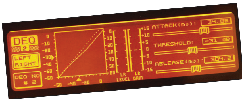
Photo 2: The DEQ function's second page provides input screens showing the attack and release times.
